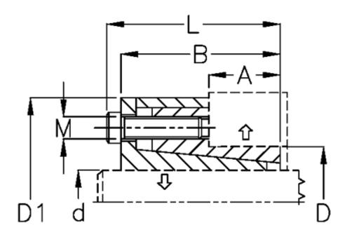
A mm = 14 B mm = 27.5 D1 mm = 40.5 d H8 mm = 20 D mm = 26 F kN torque = 14 L mm = 31.5 M mm = 4 P N/mm2 surface pressure on shaft/hub = 100
